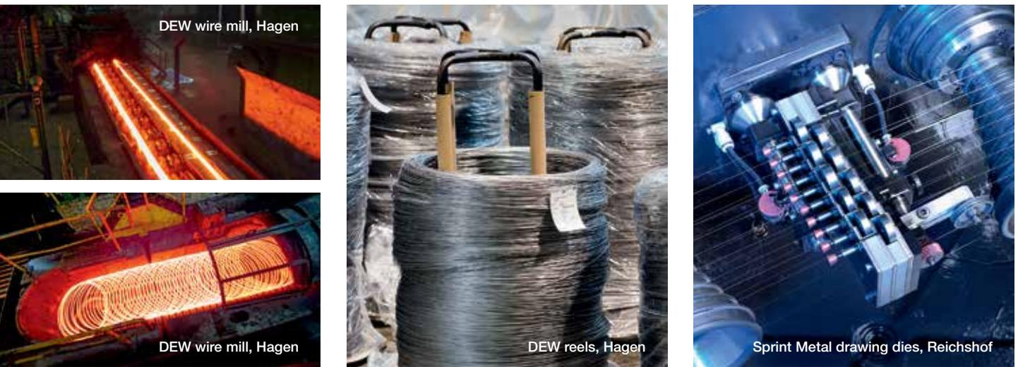
📷 *left* The 135 mm square billets are sent to the Hagen plant for further processing at the [wire mill](#). Several stands with carbide rolls make short work of the billets, producing 5.50 mm wire in a hot rolling forming process. Applying consistent volume, the 8 m billets are transformed into approx. 5 km of rolled wire at a final rolling speed of approx. 60 m/s (250 km/h).
