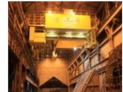
150 metric ton tapping crane (Swiss Steel)
